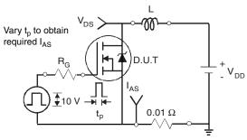
Fig. 12a - Unclamped Inductive Test Circuit
