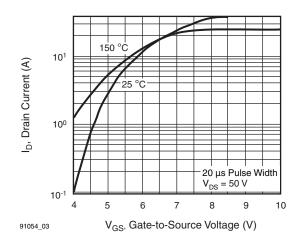
Fig. 3 - Typical Transfer Characteristics
