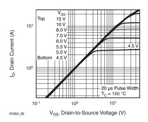
Fig. 2 - Typical Output Characteristics,  $T_C = 150 \ ^{\circ}C$
