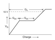
Fig. 13a - Basic Gate Charge Waveform
