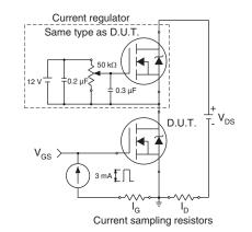
Fig. 13b - Gate Charge Test Circuit
